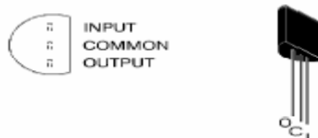
SELECT PACKAGE TO-92 (TOP VIEW)
